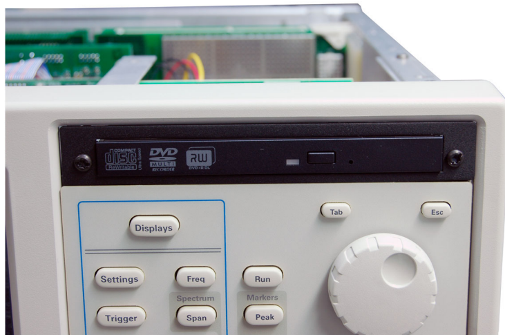
Figure 16: Installed DVD trim ring
