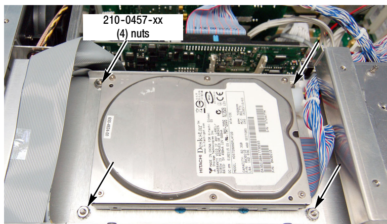
Figure 19: Securing the hard drive
